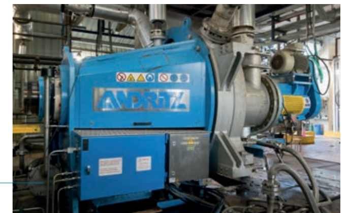
Refining is the heart of each mechanical pulping process.
